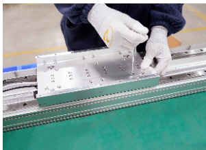
7. 滑座组装。 Slide seat assembly.
