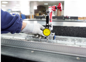
5. 检查导轨平行度。 Check the parallelism of guide rails.
