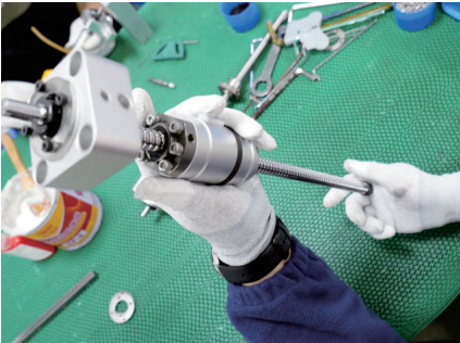
Check for any stuck condition.
