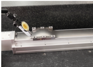
8. 通电测试重复定位精度。 Test the accuracy of repeated positioning by electrifying.
